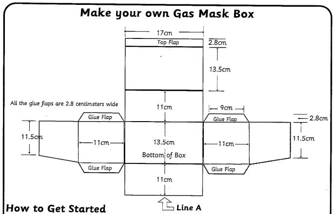
Take a large sheet of stiff brown card and draw out the net shown above to the right size. Mark the middle of the bottom edge of the card and place the centre of Line A there. Continue to draw the rest of the net and carefully cut it out. Score along the remaining lines as they are folds. Fold up your box and glue the Glue Flaps, they go inside the long sides of the box. The Top Lip tucks into the box and holds the top shut. Cut out the instructions below and stick them inside the lid.
